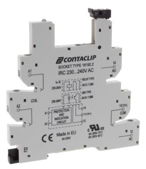
Interface-Relay-Compact (IRC) socket base IRC with screw connection, Mounting type: Mounting rail TS 35, 1 CO contact, Input voltage: 230 to 240 VAC/DC
