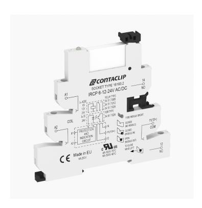
Interface-Relay-Compact (IRC) socket base IRCP with screw connection, Mounting type: Mounting rail TS 35, 1 CO contact, Input voltage: 60 VAC/DC
