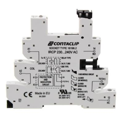
Interface-Relay-Compact (IRC) socket base IRCP with screw connection, Mounting type: Mounting rail TS 35, 1 CO contact, Input voltage: 230 to 240 VAC/DC
