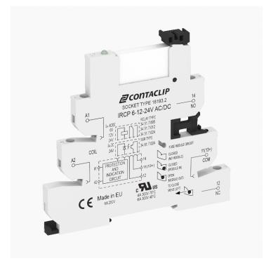
Interface-Relay-Compact (IRC) socket base IRCP with screw connection, Mounting type: Mounting rail TS 35, 1 CO contact, Input voltage: 220 VDC
