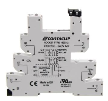
Interface-Relay-Compact (IRC) socket base IRCI with screw connection, Mounting type: Mounting rail TS 35, 1 CO contact, Input voltage: 230 to 240 VAC/DC
