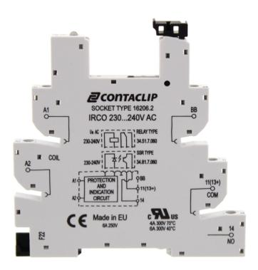
Interface-Relay-Compact (IRC) socket base IRCO with screw connection, Mounting type: Mounting rail TS 35, 1 CO contact, Input voltage: 230 to 240 VAC/DC
