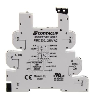
Interface-Relay-Compact (IRC) socket base FIRC with Push-In connection, Mounting type: Mounting rail TS 35, 1 CO contact, Input voltage: 230 to 240 VAC/DC
