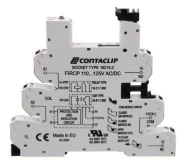
Interface-Relay-Compact (IRC) socket base FIRC P with Push-In connection, Mounting type: Mounting rail TS 35, 1 CO contact, Input voltage: 110 to 125 VAC/DC
