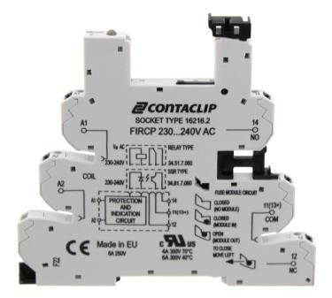
Interface-Relay-Compact (IRC) socket base FIRC P with Push-In connection, Mounting type: Mounting rail TS 35, 1 CO contact, Input voltage: 230 to 240 VAC/DC
