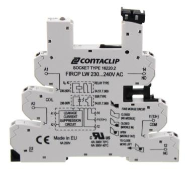
Interface-Relay-Compact (IRC) socket base FIRC P with Push-In connection and residual current suppression for long cables, Mounting type: Mounting rail TS 35, 1 CO contact, Input voltage: 230 to 240 VAC/DC
