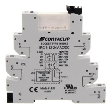
Interface-Relay-Compact (IRC) Complete, Consisting of base IRC... with screw connection and pluggable miniature relay PRC... with power contact, Mounting type: Mounting rail TS 35, 1 CO contact, Input voltage: 6 VAC/DC
