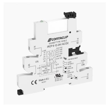
Interface-Relay-Compact (IRC) Complete, Consisting of base IRCP... with screw connection and pluggable miniature relay PRC... with power contact, Mounting type: Mounting rail TS 35, 1 CO contact, Input voltage: 60 VAC/DC
