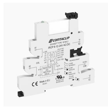
Interface-Relay-Compact (IRC) Complete, Consisting of base IRCP... with screw connection and pluggable miniature relay PRC... with power contact, Mounting type: Mounting rail TS 35, 1 CO contact, Input voltage: 125 VAC/DC
