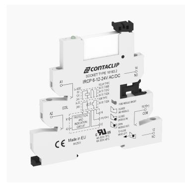
Interface-Relay-Compact (IRC) Complete, Consisting of base IRCP... with screw connection and pluggable miniature relay PRC... with power contact, Mounting type: Mounting rail TS 35, 1 CO contact, Input voltage: 240 VAC
