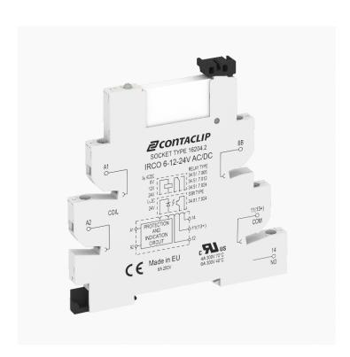
Interface-Relay-Compact (IRC) Complete, Consisting of base IRCO... with screw connection and pluggable miniature relay PRC... with power contact, Mounting type: Mounting rail TS 35, 1 CO contact, Input voltage: 6 VAC/DC
