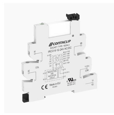
Interface-Relay-Compact (IRC) Complete, Consisting of base IRCO... with screw connection and pluggable miniature relay PRC... with power contact, Mounting type: Mounting rail TS 35, 1 CO contact, Input voltage: 240 VAC
