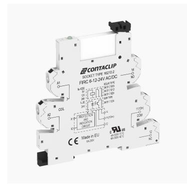
Interface-Relay-Compact (IRC) Complete, Consisting of base FIRC... with Push-In connection and pluggable miniature relay with power contact, Mounting type: Mounting rail TS 35, 1 CO contact, Input voltage: 12 VAC/DC
