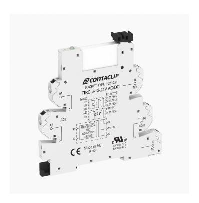
Interface-Relay-Compact (IRC) Complete, Consisting of base FIRC... with Push-In connection and pluggable miniature relay with power contact, Mounting type: Mounting rail TS 35, 1 CO contact, Input voltage: 125 VAC/DC
