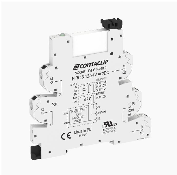
Interface-Relay-Compact (IRC) Complete, Consisting of base FIRC... with Push-In connection and pluggable miniature relay with power contact, Mounting type: Mounting rail TS 35, 1 CO contact, Input voltage: 240 VAC
