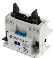
Plug adapter for Interface-Relay-Compact (IRC), ribbon plug-in connector, 14-poles, according to IEC 60603-13, for 8 relay channels, Positive switching, Rated voltage: 24 VDC
