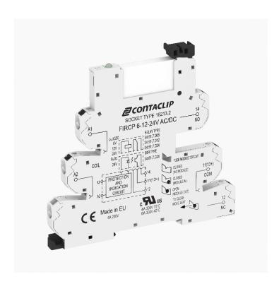
Interface-Relay-Compact (IRC) Complete, Consisting of base FIRCP... with Push-In connection and pluggable miniature relay with power contact, Mounting type: Mounting rail TS 35, 1 CO contact, Input voltage: 6 VAC/DC
