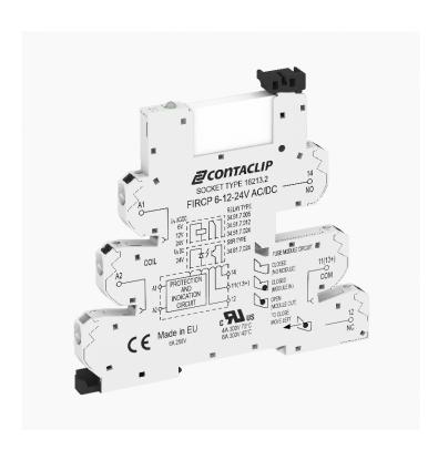
Interface-Relay-Compact (IRC) Complete, Consisting of base FIRCP... with Push-In connection and pluggable miniature relay with power contact, Mounting type: Mounting rail TS 35, 1 CO contact, Input voltage: 24 VAC/DC
