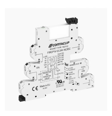
Interface-Relay-Compact (IRC) Complete, Consisting of base FIRCP... with Push-In connection and pluggable miniature relay with power contact, Mounting type: Mounting rail TS 35, 1 CO contact, Input voltage: 240 VAC
