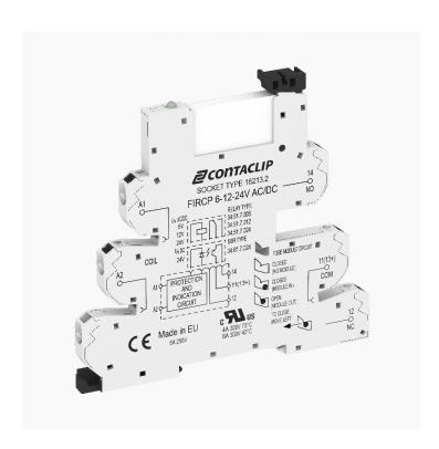
Interface-Relay-Compact (IRC) Complete, Consisting of base FIRCP... with Push-In connection and pluggable miniature relay with power contact, Mounting type: Mounting rail TS 35, 1 CO contact, Input voltage: 125 VDC
