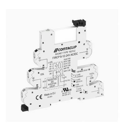
Interface-Relay-Compact (IRC) Complete, Consisting of base FIRCP... with Push-In connection and pluggable miniature relay with power contact, Mounting type: Mounting rail TS 35, 1 CO contact, Input voltage: 220 VDC
