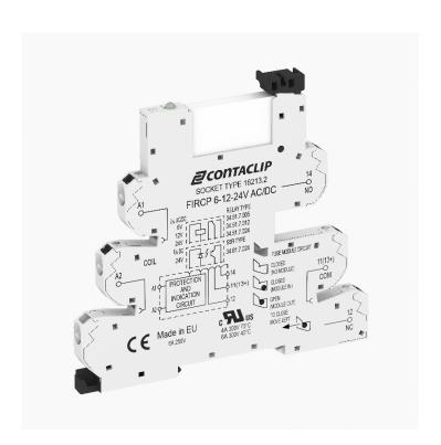
Interface-Relay-Compact (IRC) Complete, Consisting of base FIRCP... with Push-In connection and pluggable miniature relay with power contact, Mounting type: Mounting rail TS 35, 1 CO contact, Input voltage: 240 VAC
