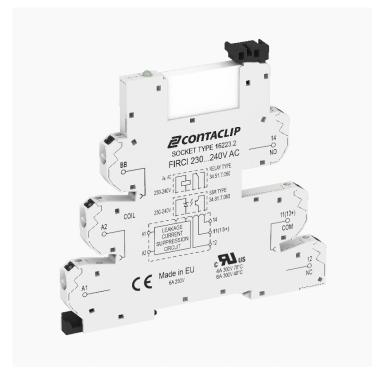
Interface-Relay-Compact (IRC) Complete, Consisting of base FIRCI... with Push-In connection and pluggable miniature relay with power contact, Mounting type: Mounting rail TS 35, 1 CO contact, Input voltage: 6 VAC/DC
