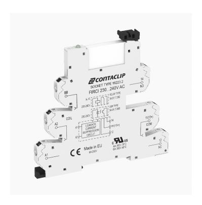
Interface-Relay-Compact (IRC) Complete, Consisting of base FIRCI... with Push-In connection and pluggable miniature relay with power contact, Mounting type: Mounting rail TS 35, 1 CO contact, Input voltage: 240 VAC
