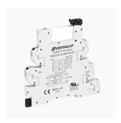
Interface-Relay-Compact (IRC) Complete, Consisting of base FIRCO... with Push-In connection and pluggable miniature relay with power contact, Mounting type: Mounting rail TS 35, 1 CO contact, Input voltage: 6 VAC/DC
