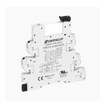
Interface-Relay-Compact (IRC) Complete, Consisting of base FIRCO... with Push-In connection and pluggable miniature relay with power contact, Mounting type: Mounting rail TS 35, 1 CO contact, Input voltage: 12 VAC/DC
