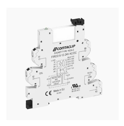
Interface-Relay-Compact (IRC) Complete, Consisting of base FIRCIO... with Push-In connection and pluggable miniature relay with power contact, Mounting type: Mounting rail TS 35, 1 CO contact, Input voltage: 24 VAC/DC
