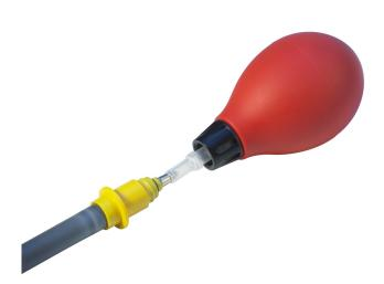
If the pen has writing problems, the tip of the pen can be sucked free with the help of the pressure ball. The pressure ball is compressed and then placed on the plotter pen tip. After the bulb is released, the vacuum created in the bulb sucks the pen tip free.
