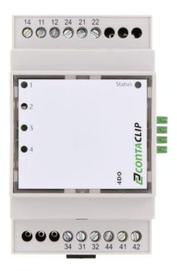
GSM-PRO I/O digital output module, 4 relay outputs 1 W, 250 V, 16 A (inrush 80 A), With LED display, Mounting type: Mounting rail TS 35, Supply voltage range: 20 - 28 VDC
