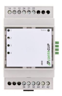
GSM-PRO I/O digital output module, 4 relay outputs 1 W, 250 V, 16 A (inrush 80 A), With LED display, Mounting type: Mounting rail TS 35, Supply voltage: 12 VDC
