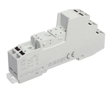
Relay socket base PRS, for miniature power relay with 2 CO contacts, Push-in connection, Plug-in option for input/suppression modules and cross connections, Mounting type: Mounting rail TS 35
