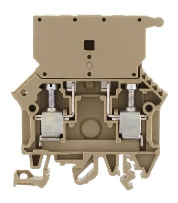
Fused terminal with disconnect plug, Screw connection, Mounting type:Mounting rail TS 35/7.5 and TS 32, Rated cross-section: 10 mm², Width: 8 mm, Colour: Beige
