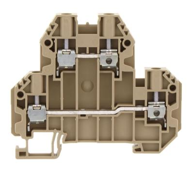
Double-level terminal, Screw connection, Mounting type: Mounting rail TS 35/7.5, Rated cross-section: 4 mm², Width: 6.1 mm, Colour: Beige
