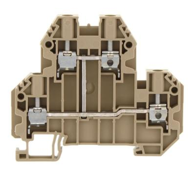
Double-level terminal, Screw connection, Mounting type: Mounting rail TS 35/7.5, Rated cross-section: 4 mm², Width: 6.1 mm, Colour: Beige
