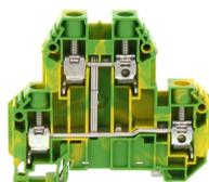
Protective-earth double-level terminal, Screw connection, Mounting type: Mounting rail TS 35/7.5, Rated cross-section: 10 mm<sup>2</sup>, Width: 10.1 mm, Colour: Green-yellow
