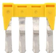
Insulated cross-connector, No. of poles: 4, Mounting type: Plug in, Width: 23.5 mm, Rated cross-section: 4 mm<sup>2</sup>, Colour: Yellow
