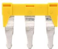
Insulated cross-connector, No. of poles: 3, Mounting type: Plug in, Width: 27.6 mm, Rated cross-section: 10 mm<sup>2</sup>, Colour: Yellow
