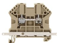
Feed-through terminal, Screw connection, Mounting type: Mounting rail TS 35/7.5, Rated cross-section: 2.5 mm<sup>2</sup>, Width: 5 mm, Colour: Beige
