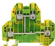
Protective-earth double-level terminal, Screw connection, Mounting type: Mounting rail TS 35/7.5, Rated cross-section: 4 mm<sup>2</sup>, Width: 6.1 mm, Colour: Green-yellow
