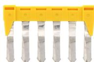
Insulated cross-connector, No. of poles: 6, Mounting type: Plug in, Width: 35.7 mm, Rated cross-section: 4 mm<sup>2</sup>, Colour: Yellow
