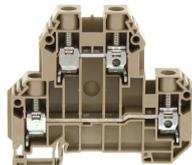
Double-level terminal, Screw connection, Mounting type: Mounting rail TS 35/7.5, Rated cross-section: 10 mm<sup>2</sup>, Width: 10.1 mm, Colour: Beige
