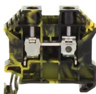
Feed-through terminal, Screw connection, Mounting type: Mounting rail TS 35/7.5, Rated cross-section: 16 mm<sup>2</sup>, Width: 10 mm, Colour: Black-yellow
