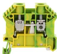
Protective earth terminal, Screw connection, Mounting type: Mounting rail TS 35/7.5, Rated cross-section: 16 mm<sup>2</sup>, Width: 10 mm, Colour: Green-yellow
