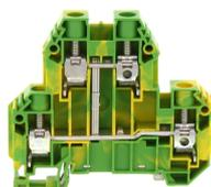
Protective-earth double-level terminal, Screw connection, Mounting type: Mounting rail TS 35/7.5, Rated cross-section: 10 mm<sup>2</sup>, Width: 10.1 mm, Colour: Green-yellow
