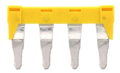
Insulated cross-connector, No. of poles: 4, Mounting type: Plug in, Width: 37.7 mm, Rated cross-section: 10 mm², Colour: Yellow
