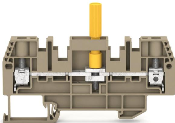
Test disconnect terminal, Screw connection, Mounting type: Mounting rail TS 35/7.5, Rated cross-section: 6 mm<sup>2</sup>, Width: 8.1 mm, Colour: Beige
