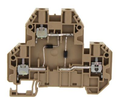
Double-level terminal with electronic components, Screw connection, Mounting type:Mounting rail TS 35/7.5, Rated cross-section: 4 mm², Width: 6.1 mm, Colour: Beige
