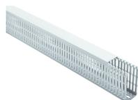
Cabling duct, Mounting type: Adhere, Width: 25 mm, Height: 40 mm, Material: PC-ABS, Colour: Light grey
