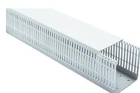
Cabling duct with cover, Mounting type: Rivets, Width: 60 mm, Height: 40 mm, Material: PC-ABS, Colour: Light grey
