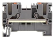
Feed-through terminal, Push-in connection, Mounting type: Mounting rail TS 35/7.5, Rated cross-section: 2.5 mm<sup>2</sup>, Width: 5.1 mm, Colour: Grey
