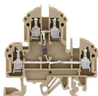
Double-level terminal with electronic components, Screw connection, Mounting type: Mounting rail TS 35/7.5 and TS 32, Rated cross-section: 4 mm<sup>2</sup>, Width: 6 mm, Colour: Beige
