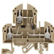
Double-level terminal with electronic components, Screw connection, Mounting type: Mounting rail TS 35/7.5 and TS 32, Rated cross-section: 4 mm<sup>2</sup>, Width: 6 mm, Colour: Beige
