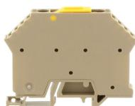
Disconnect terminal, Screw connection, Mounting type: Mounting rail TS 15/5.5, Rated cross-section: 2.5 mm<sup>2</sup>, Width: 6 mm, Colour: Beige
