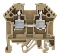
Ex feed-through terminal ATEX-certified, Screw connection, Mounting type: Mounting rail TS 35/7.5 and TS 32, Rated cross-section: 4 mm<sup>2</sup>, Width: 6 mm, Colour: Beige
