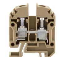
Ex feed-through terminal ATEX-certified, Screw connection, Mounting type: Mounting rail TS 15/5.5, Rated cross-section: 4 mm<sup>2</sup>, Width: 6 mm, Colour: Beige
