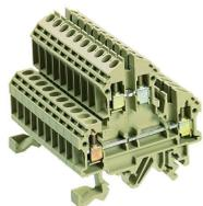
Double-level terminal/block variant, Screw connection, Mounting type: Mounting rail TS 35/7.5 and TS 32, Rated cross-section: 4 mm<sup>2</sup>, Colour: Beige
