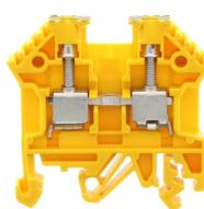
Feed-through terminal, Screw connection, Mounting type: Mounting rail TS 35/7.5 and TS 32, Rated cross-section: 4 mm<sup>2</sup>, Width: 6 mm, Colour: Black-yellow
