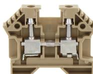
Feed-through terminal for direct mount/block variant, Screw connection, Mounting type: Mounting surface, Rated cross-section: 4 mm<sup>2</sup>, Width: 6 mm, Colour: Beige
