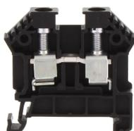
Feed-through terminal, Screw connection, Mounting type: Mounting rail TS 35/7.5, Rated cross-section: 10 mm<sup>2</sup>, Width: 8 mm, Colour: Black
