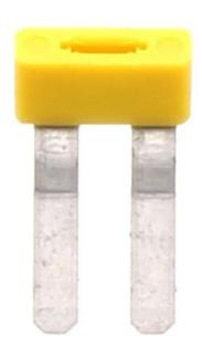
External insulated cross-connector, No. of poles: 2, Mounting type: Plug in, Width: 9.26 mm, Rated current: 27 A; Colour: Yellow
