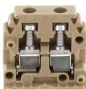
Feed-through terminal for direct mount, Screw connection, Mounting type: Mounting surface, Rated cross-section: 2.5 mm<sup>2</sup>, Width: 5 mm, Colour: Beige
