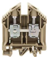
Feed-through terminal, Screw connection, Mounting type: Mounting rail TS 35/7.5 and TS 32, Rated cross-section: 35 mm<sup>2</sup>, Width: 16 mm, Colour: Beige
