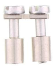
Cross-connector, No. of poles: 2, Mounting type: Can be screwed on, Width: 9.1 mm, Rated cross-section: 2.5 mm², Colour: natural
